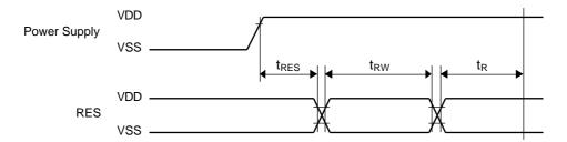
All signal timings are based on 20% and 80% of  $V_{\rm DD}$  signals.
